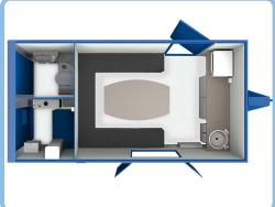
Mobile and secure, the Border Eco Cabin comprises a 6-person canteen, private toilet facilities and a drying/changing/generator room, making it ideal for even the most challenging site locations.
